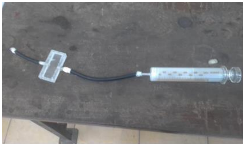
Figure 1: Pictorial diagram of customized gas chamber
