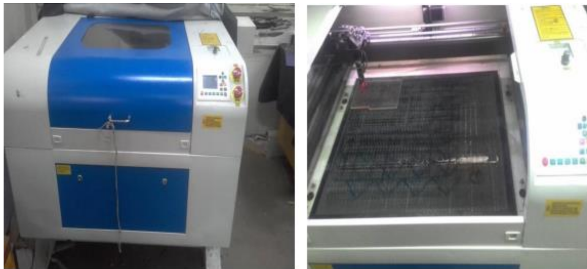
Figure 2: Pictorial diagrams of a laser engraving machine
