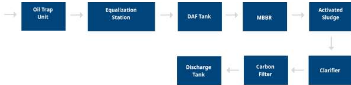
Figure 1: POME Water Treatment Plant Process Flow Diagram
