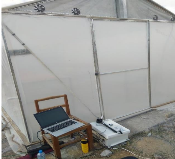
Figure 4. Computer, data logger and instruments for recording drying data
