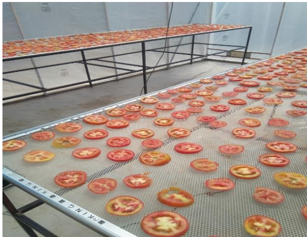
Figure 2. The inside of the Greenhouse Solar Dryer showing the sliced tomato on drying trays
