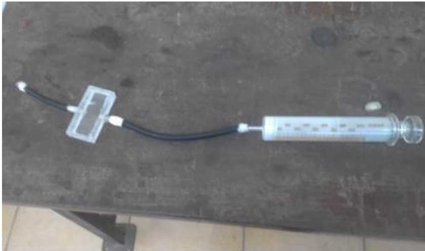
Figure 1: Pictorial diagram of customized gas chamber
