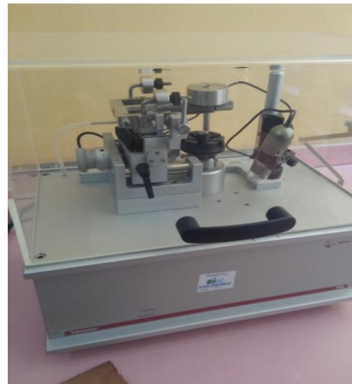
Plate 4: Tribometer for wear test
